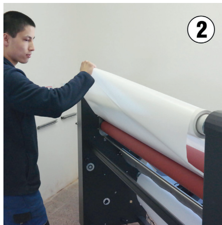
2 Hold the inserted laminate in place tightly and close the rollers
